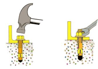
2. Place nut on the end of the wedge anchor (to protect the threads of the wedge anchor during installation) Drive wedge anchor into drilled hole up) anchorage is now complete. through fixture so that nut is flush with fixture.
