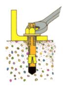
2. Place nut on the end of the wedge anchor (to protect the threads of the wedge anchor during installation) Drive wedge anchor into drilled hole up) anchorage is now complete. through fixture so that nut is flush with fixture.
